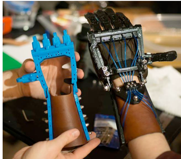
Figure 1. An example of a 3D-printable prosthetic hand, a popular type of assistive technology featured on Thingiverse.com. (Thing # 229620)
