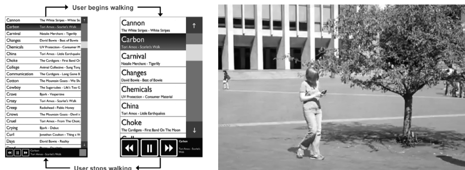
Fig. 9. Our walking user interface adapts to a user’s situationally-impaired visual and motor abilities. When the user begins walking, the on-screen text and targets increase in size. On the right, a participant in our user study is shown walking an outdoor course with our mobile device. Although our prototype detected standing vs. walking using the device’s camera, for our study we simulated adaptation using the Wizard-of-Oz technique.
