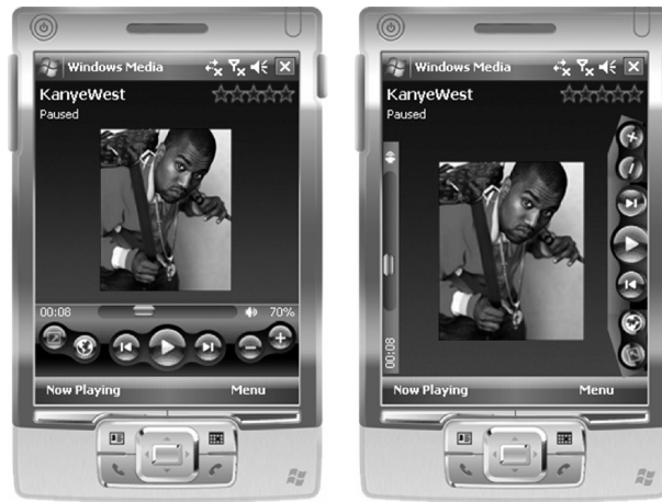
Fig. 8. The left design is a typical music player, with targets near the screen bottom in “open space.” The right design has targets along the left and right screen edges, where elevated physical bezels improve accuracy when used in conjunction with the lift-off selection technique. Although round, the right-side targets would be made responsive all the way to the screen edge.
